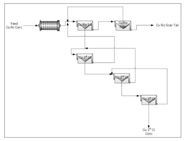
The main objective of tests LCT-7 and LCT-8 was to generate Cu/Ni cleaner concentrates. The Cu/Ni cleaner concentrates were filtered and the total wet weight was recorded. A subsample was taken for moisture measurement and assay. The remaining sample was repulped and stored until a Cu-Ni separation test could be performed.
