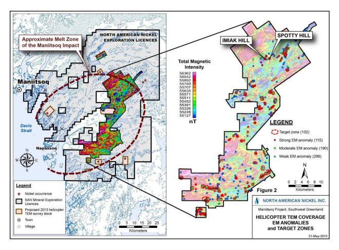
**Figure 2**: Plan map of the Maniitsoq project showing helicopter TEM coverage (area covered by colour magnetic images) and exploration target zones.
