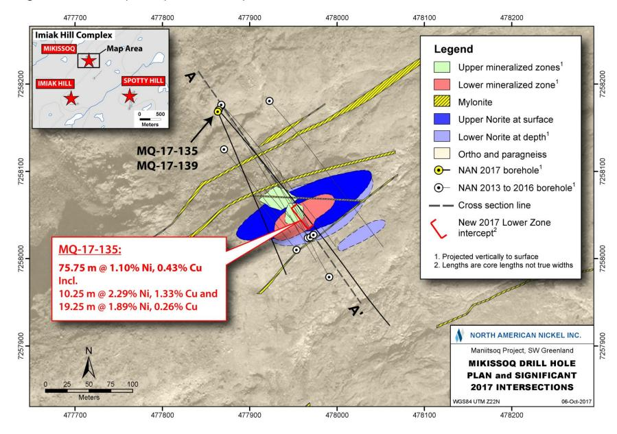
Figure 2: Surface drill plan map of the Mikissoq area.
